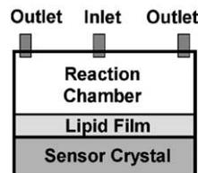
Fig. 2. The QCM-D set-up with the piezoelectric quartz crystal sensor as base in the reaction chamber. The sensor surface is circular with a diameter of 14 mm and the chamber height is  $\sim 0.5\text{ mm}$ , i.e. the chamber volume is  $\sim 80\ \mu\text{l}$ . Note that dimensions are not in correct proportions in this illustration.
