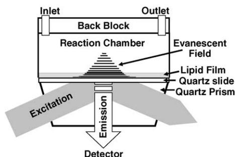
Fig. 3. Illustration of the TIRF flow cell. The volume of the reaction chamber is approximately  $3.5 \mu\text{l}$ , created by a height of  $0.01 \text{ mm}$  and a base area of approximately  $350 \text{ mm}^2$  (a rectangular shape of  $16 \text{ mm}$  broad and  $24 \text{ mm}$  long with cut edges). Note that dimensions are not in correct proportions.
