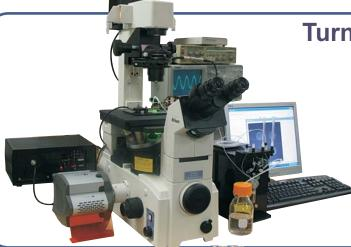
Turnkey Single Molecule Detection TIRF Microscopy Station
